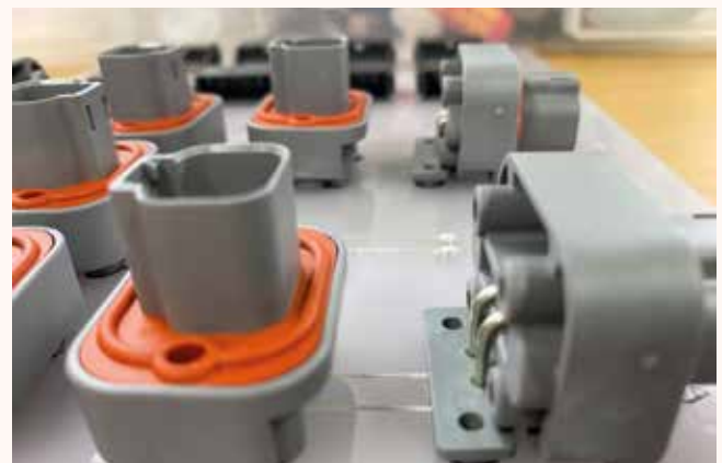
Printed conductors electrically and mechanically contacted on automotive-approved connectors.
