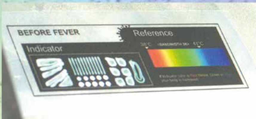
Technology demonstrator for temperature indication in fever patients by printing thermochromic inks onto skin-compatible substrates.
