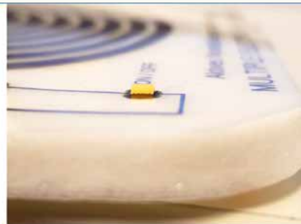
Technology demonstrator for an electrically active wound patch with printed electrodes on flexible substrates.
