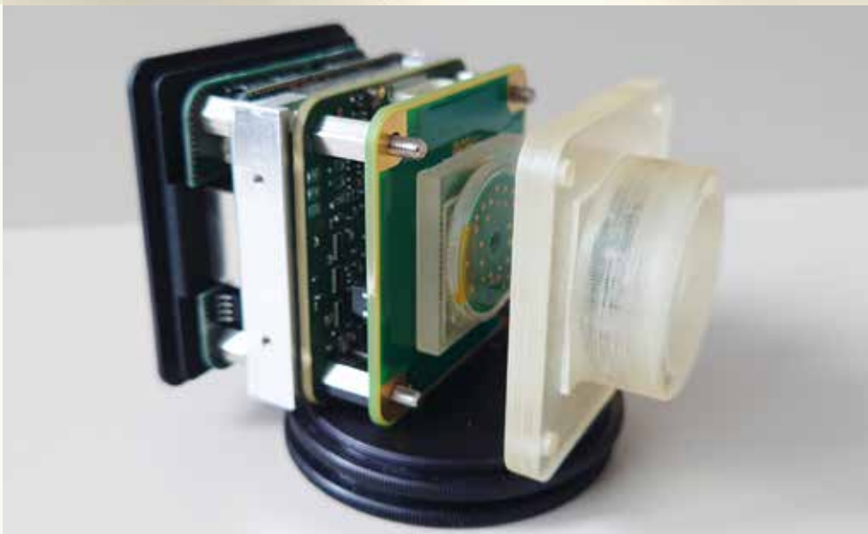
Hyperspectral camera system with Vision-System-on-Chip (VSoC) image sensor and a tunable Fabry-Pérot filter developed by Fraunhofer ENAS. (Photo © Fraunhofer IIS/EAS)
