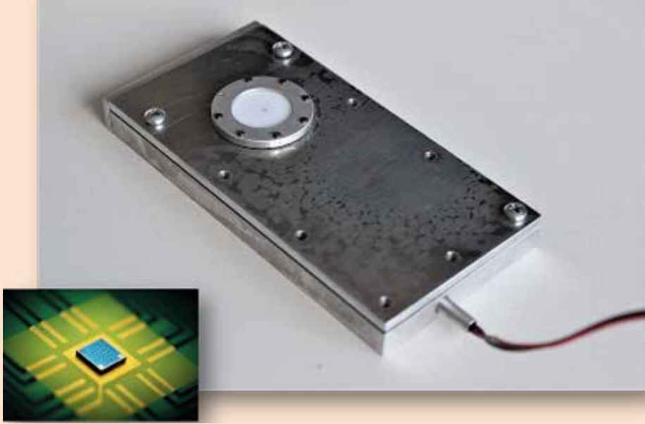
The transducer mounted on a PCB, and its housing.
